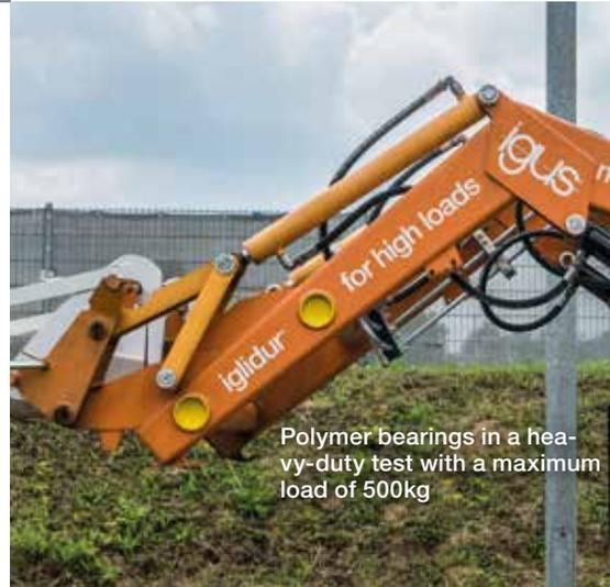
Polymer bearings in a heavy-duty test with a maximum load of 500kg
